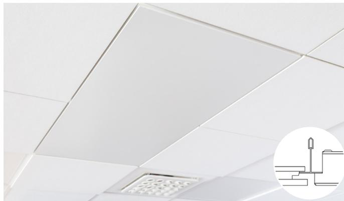
ItuGraf® Model M has been designed to match the M edge. The M edge design has concealed support edges to create a distinctive floating appearance. The suspension grid is approximately 14 mm above the visible surface of the tile, which gives the impression that each tile is individually suspended. All of the tiles are easily demountable.
