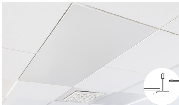
ItuGraf® Model Dg has been designed to match the Dg edge in the Focus range. The Dg edge design has concealed support edges to create a distinctive floating appearance. The suspension grid is approximately 14 mm above the visible surface of the tile, which gives the impression that each tile is individually suspended. All of the tiles are easily demountable.
